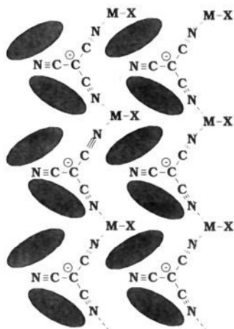
Figure 12. Materialized candidate of the anion layer which will give \kappa -type BEDT-TTF salts. For example, M = transition metal and X = halogen anion or MX = neutral molecule. The shaded parts correspond to the openings.
